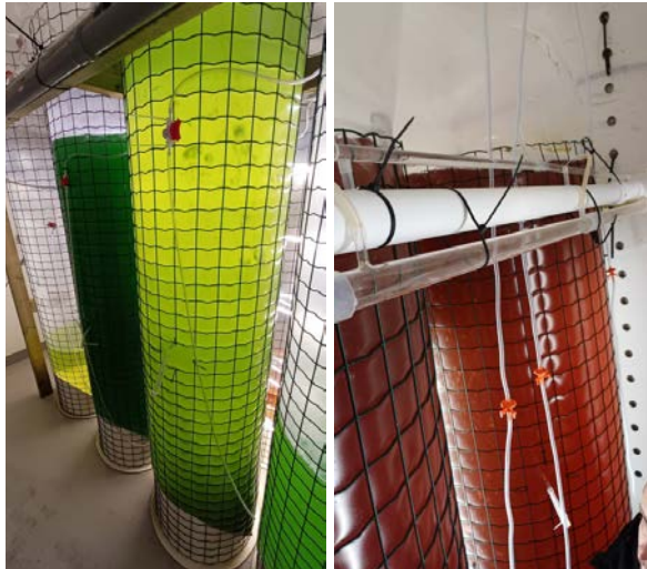
Fig. 5. Examples of plastic bags and algae cultivation systems (Photo – Olifirenko V.V.)
